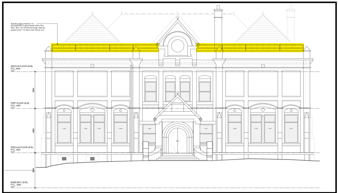
Fig.3. Proposed East Principal Elevation with guardrail
