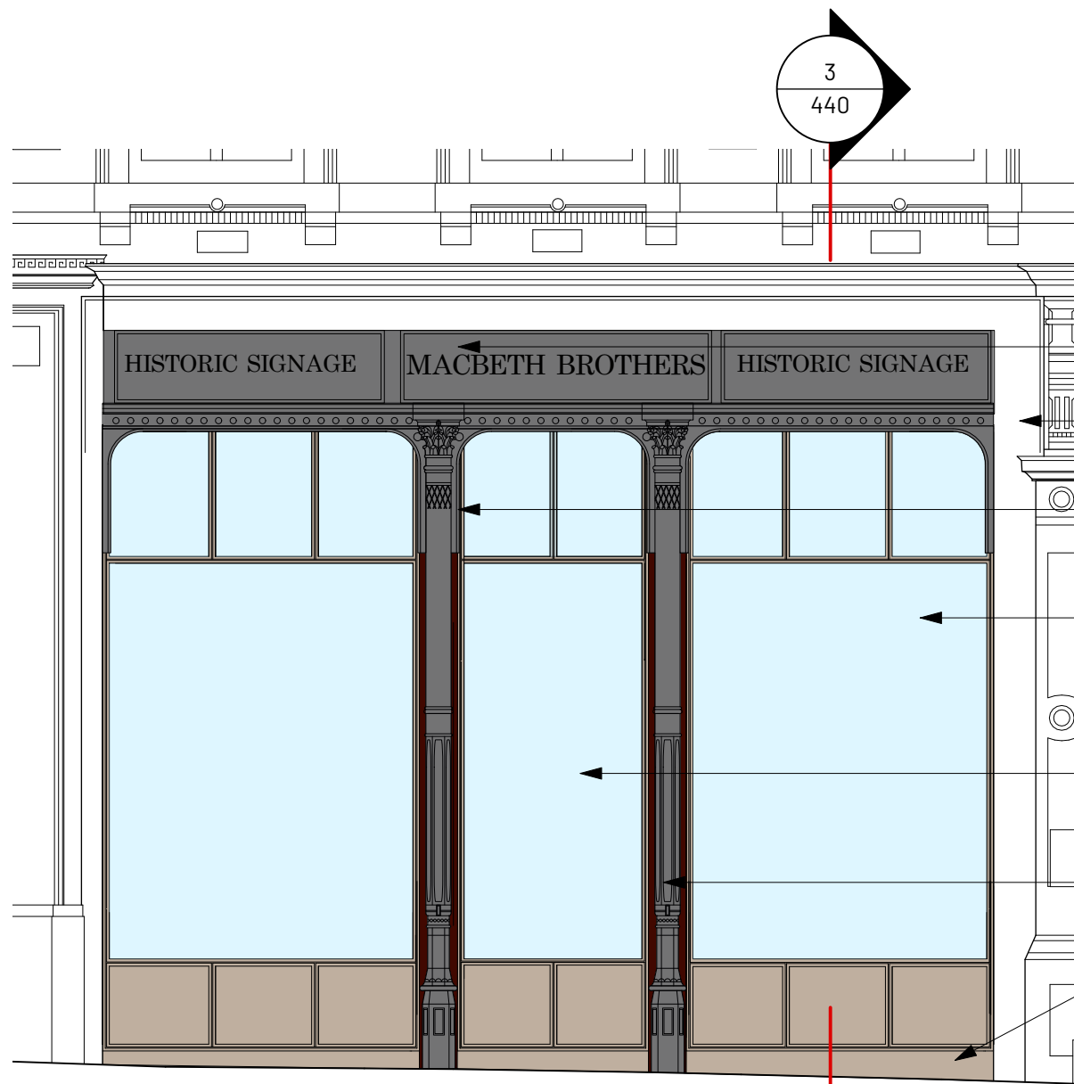
1 Proposed Shop Front Elevation Scale: 1:50
