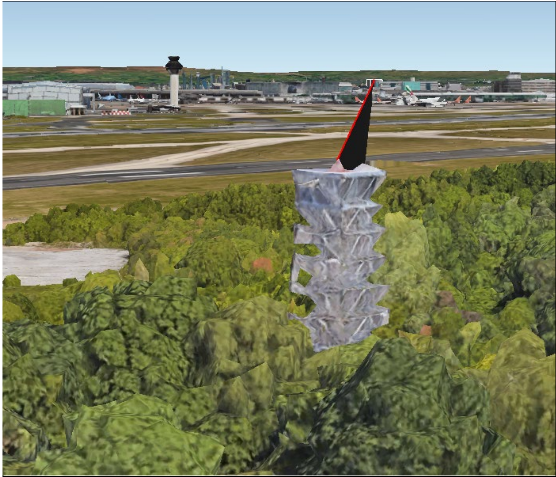
Figure 6 - A NATS provided image indicating the outline of the Proposed Development and the line-of-sight (LOS) path from Manchester Airport's SSR to the Site
