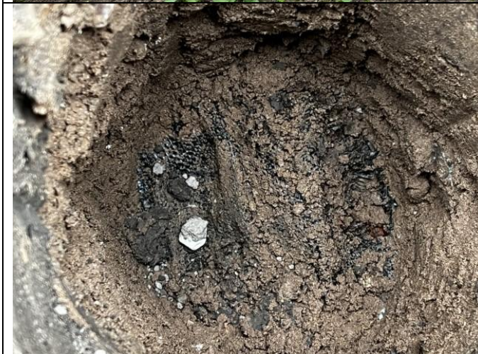
Photograph 18: View showing membrane in base of trial pit (area 6).
