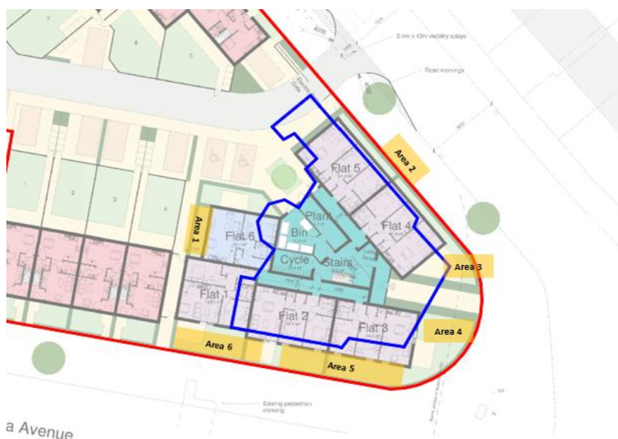
Plate 3-1: Capping layer inspection areas in apartment block soft landscaping.
