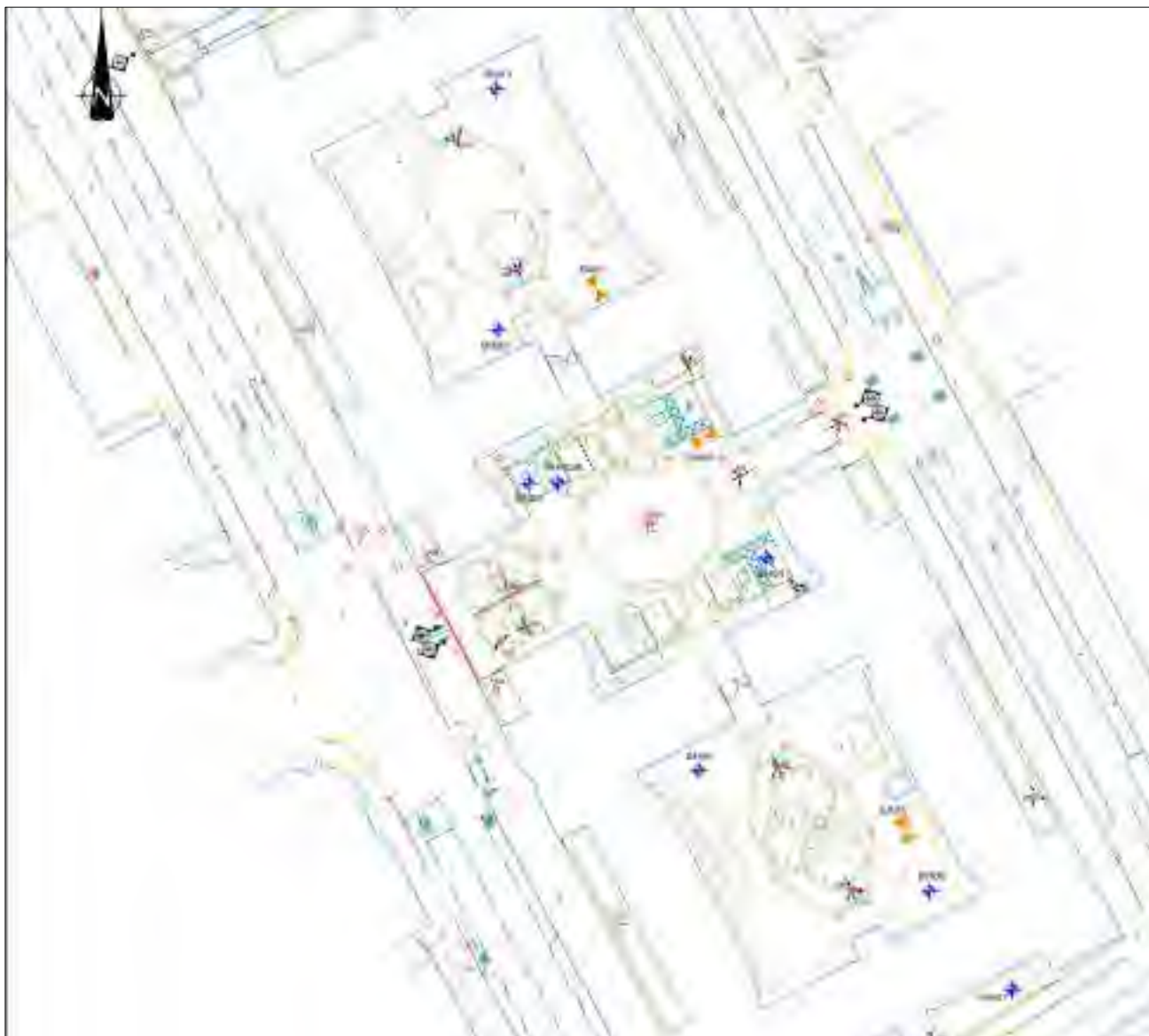
Figure 4 'As built' ground investigation locations[3]
