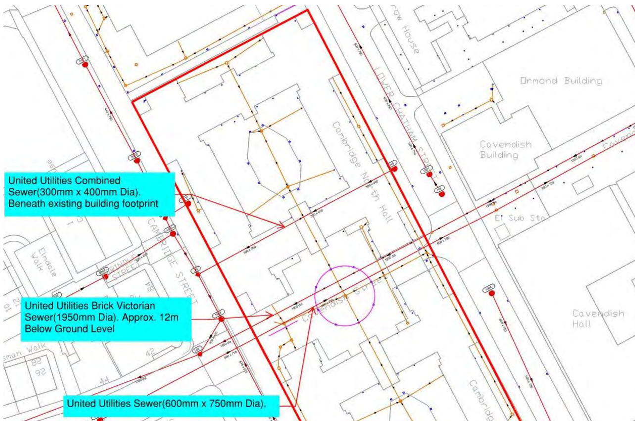
Figure 2 United Utilities assets present on site
