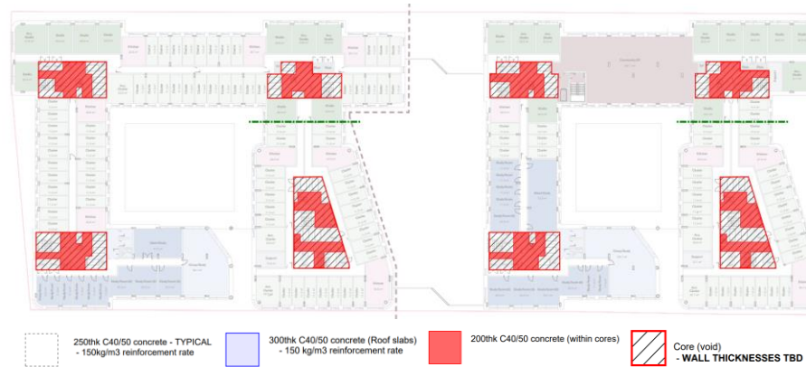
Option 1- Reinforced Concrete Flat Slab
