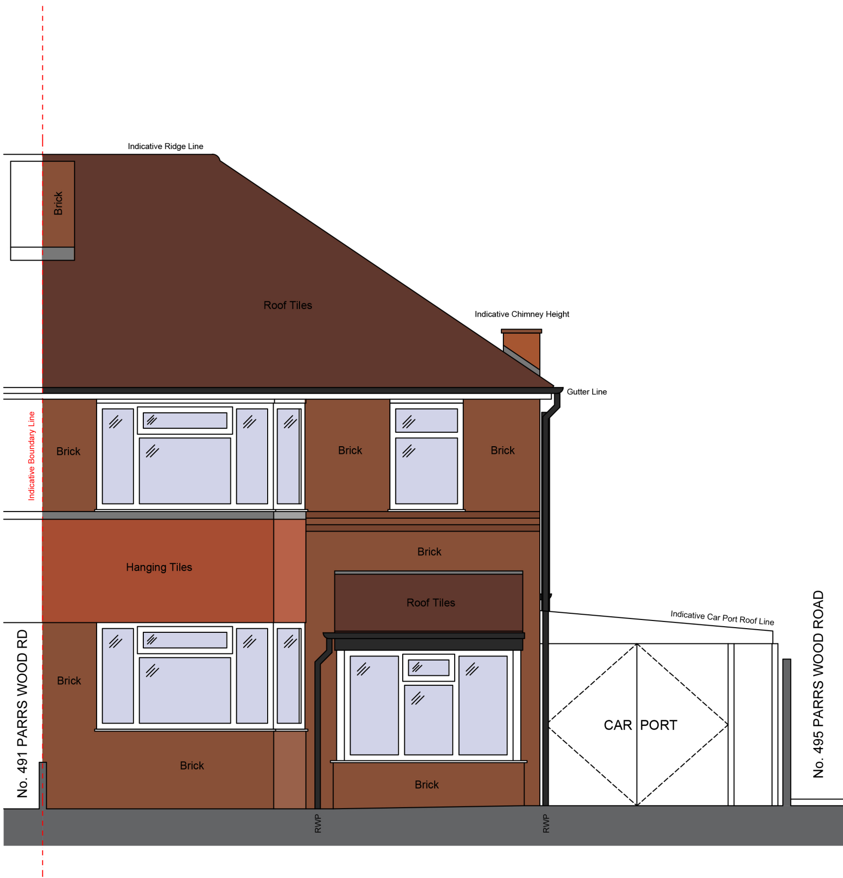
Existing North West Elevation - to Parrs Wood Road
