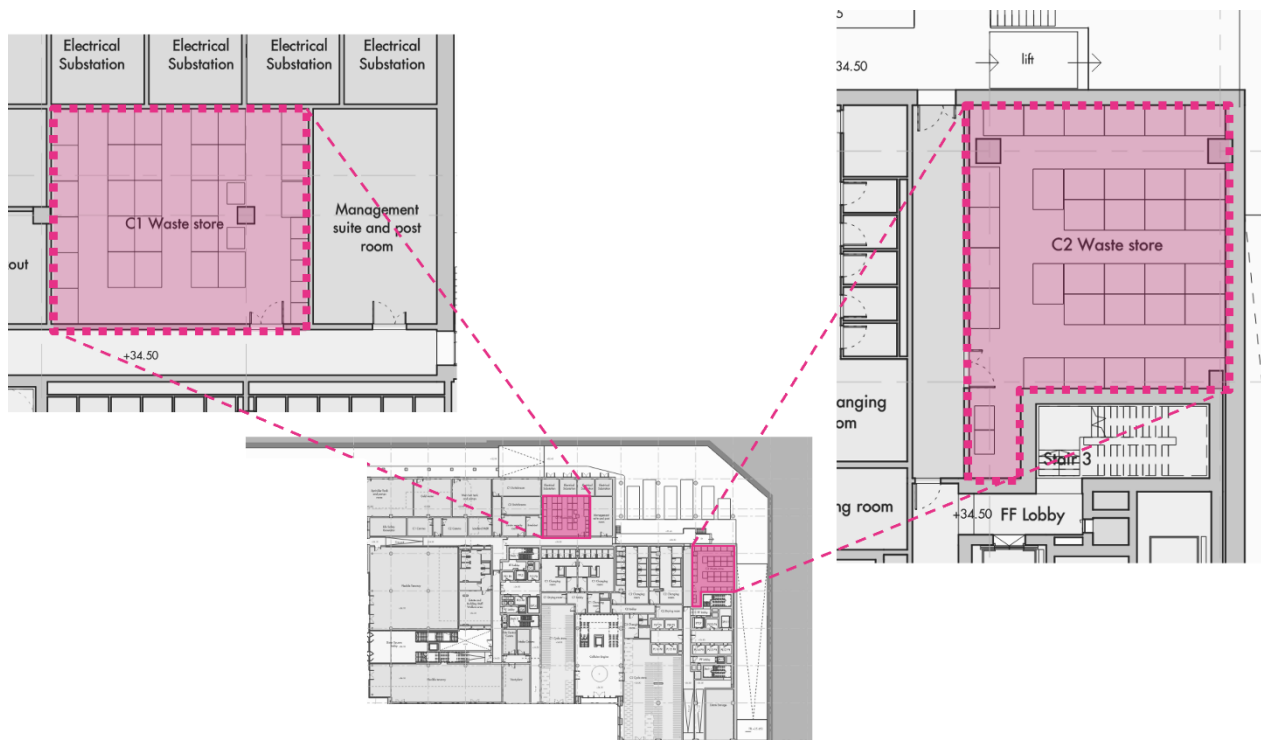
Figure 9: Operational waste storage spaces
