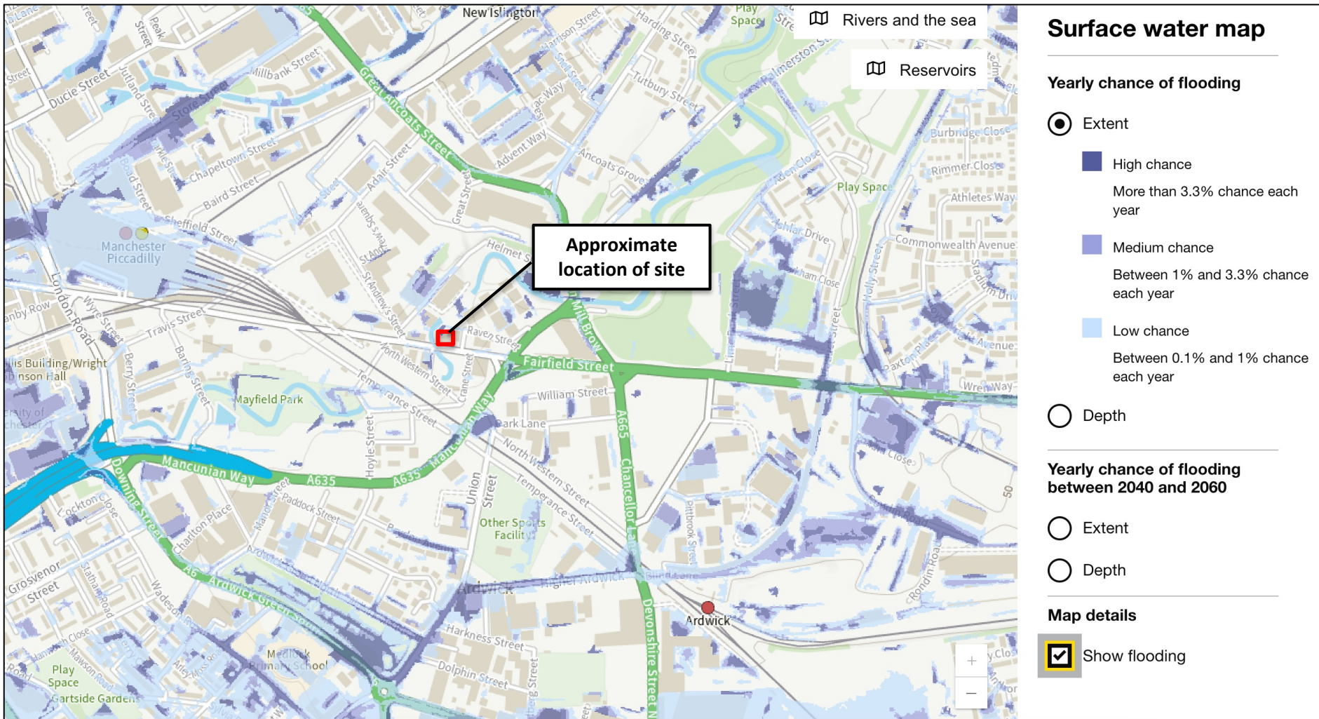
Figure 3 Environment Agency's Surface Water Flood Risk Map
