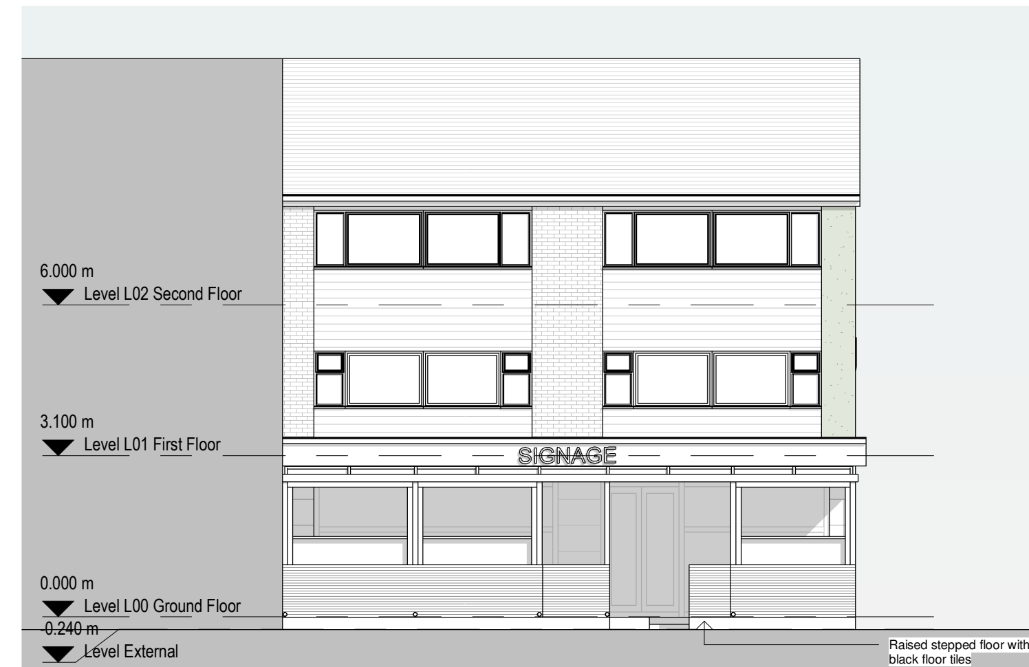
3 As-built East Elevation 1 : 100
