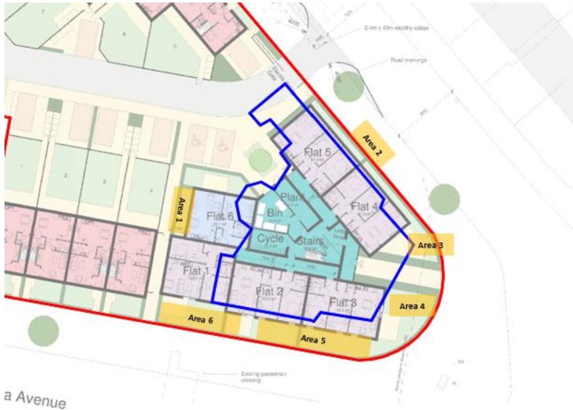
Plate 4-1: Capping layer inspection areas in apartment block soft landscaping.
