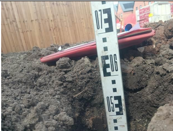
Photograph 2: Evidence of suitably chemically validated topsoil with a minimum of 150mm growing medium in rear garden areas (Plot 3) over natural strata.
