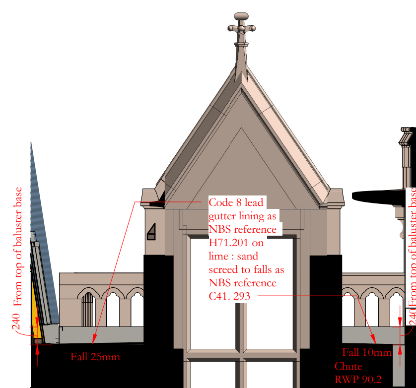
Lloyd Street courtyard east gutter roof slope CBR02
