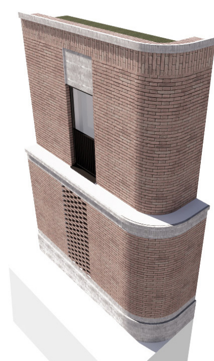
Wetcast concrete plinth, horizontal band and corner brickwork
