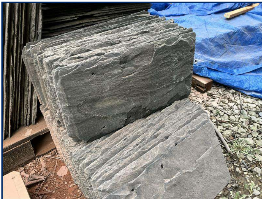
Photo [12] - Proposed Natural Welsh Slate as per the existing
