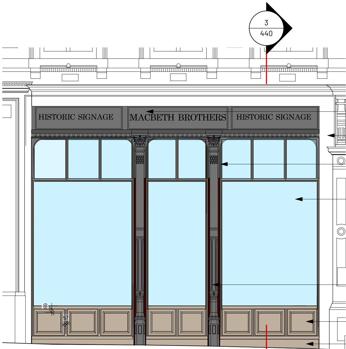
1 Proposed Shop Front Elevation Scale: 1:50
