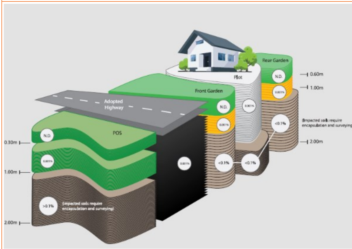
FIGURE 4.1 ASBESTOS RISK MITIGATION CONCEPTUAL SITE MODEL
