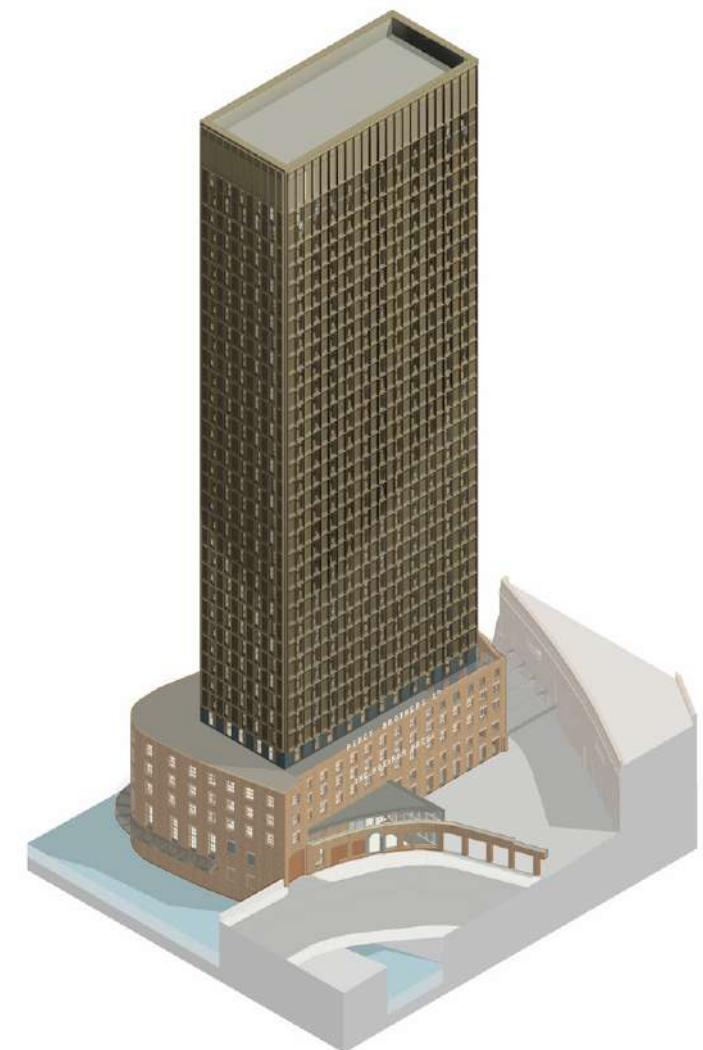
Anodised aluminium - Anolok 543, unitised facade system tower
