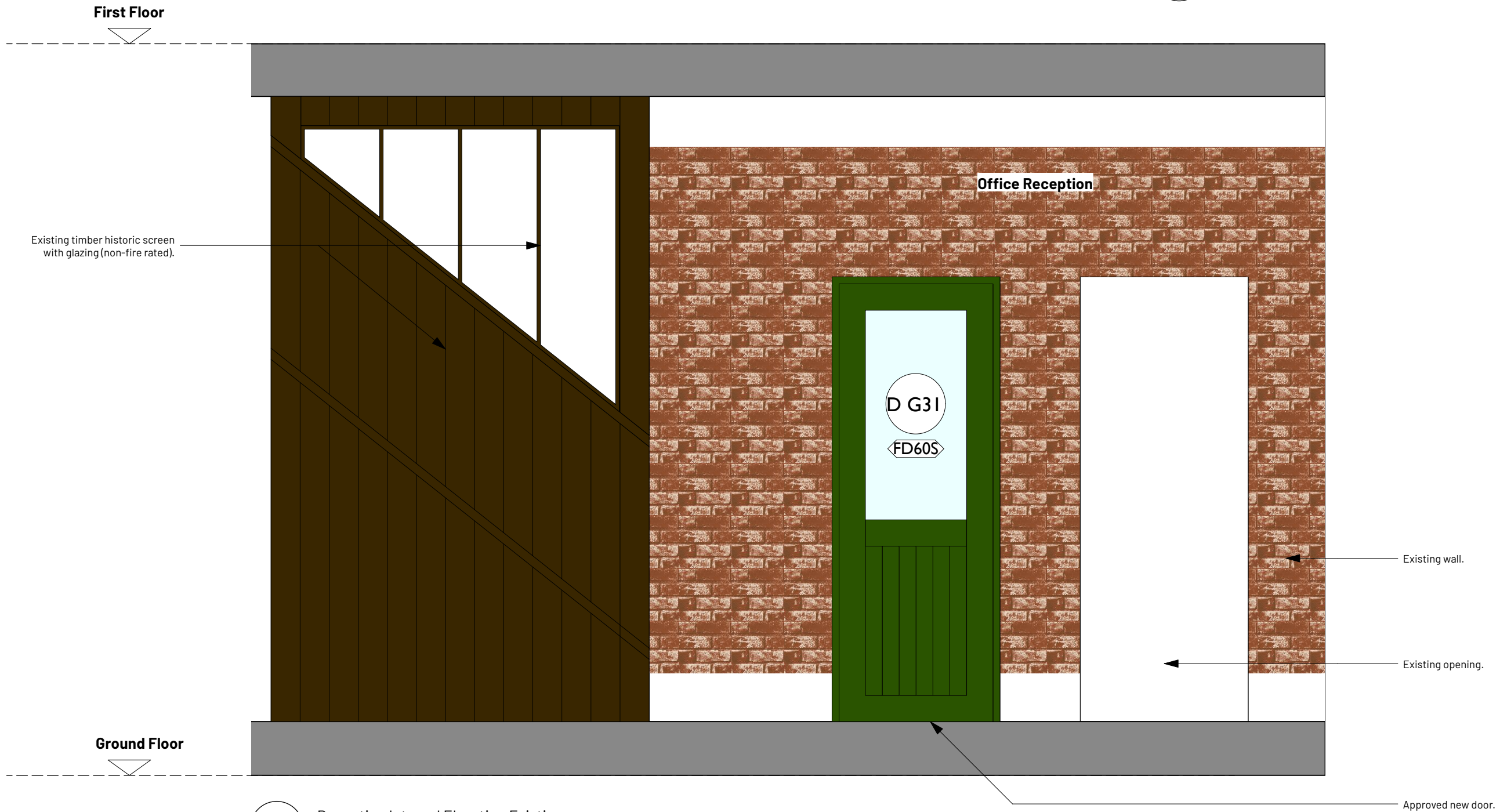
2 Reception Internal Elevation Existing Scale: 1:25
