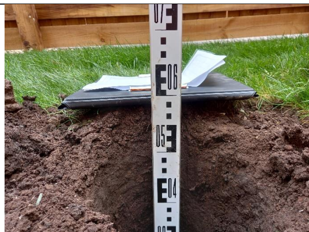
Photograph 1: Evidence of suitably chemically validated soil cover to 600mm in the rear garden of plot 9.
