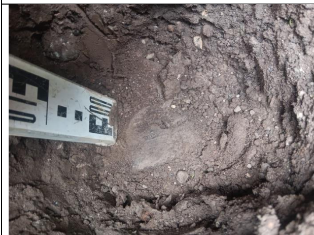
Photograph 41: Evidence of geotextile membrane in plot 17.
