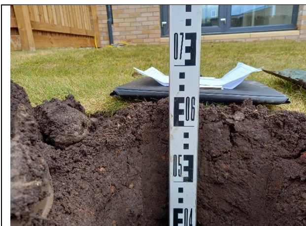
Photograph 62: Evidence of suitably chemically validated soil cover to 640mm in the rear garden of plot 22.
