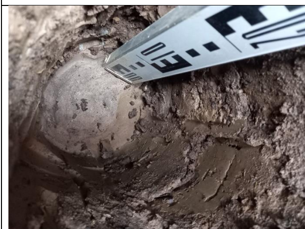
Photograph 20: Evidence of geotextile membrane in plot 13.
