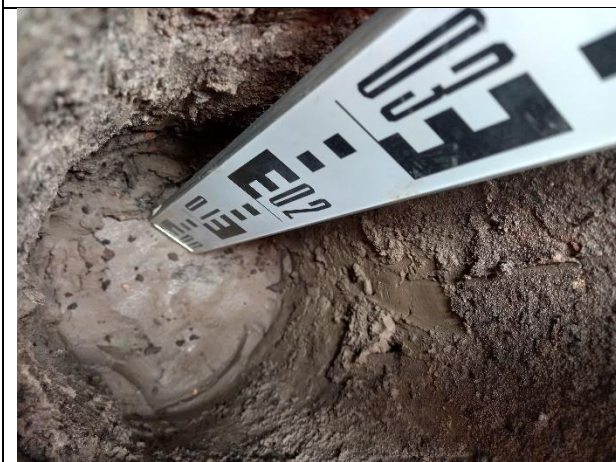
Photograph 28: Evidence of geotextile membrane in plot 14.
