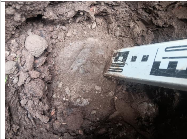
Photograph 6: Evidence of geotextile membrane in plot 10.
