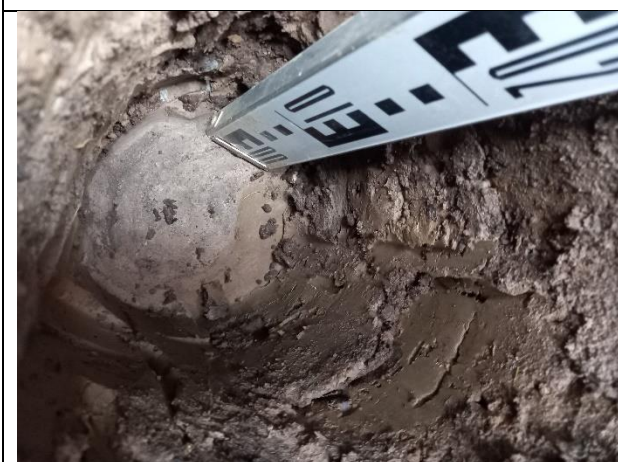
Photograph 24: Evidence of geotextile membrane in plot 13.
