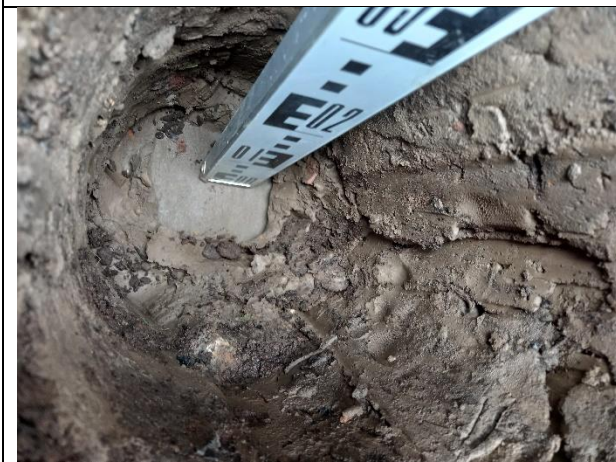
Photograph 33: Evidence of geotextile membrane in plot 15.
