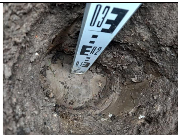
Photograph 2: Evidence of geotextile membrane in plot 9.
