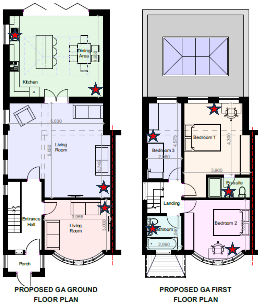
Plate 1: Internal bin potential storage locations
