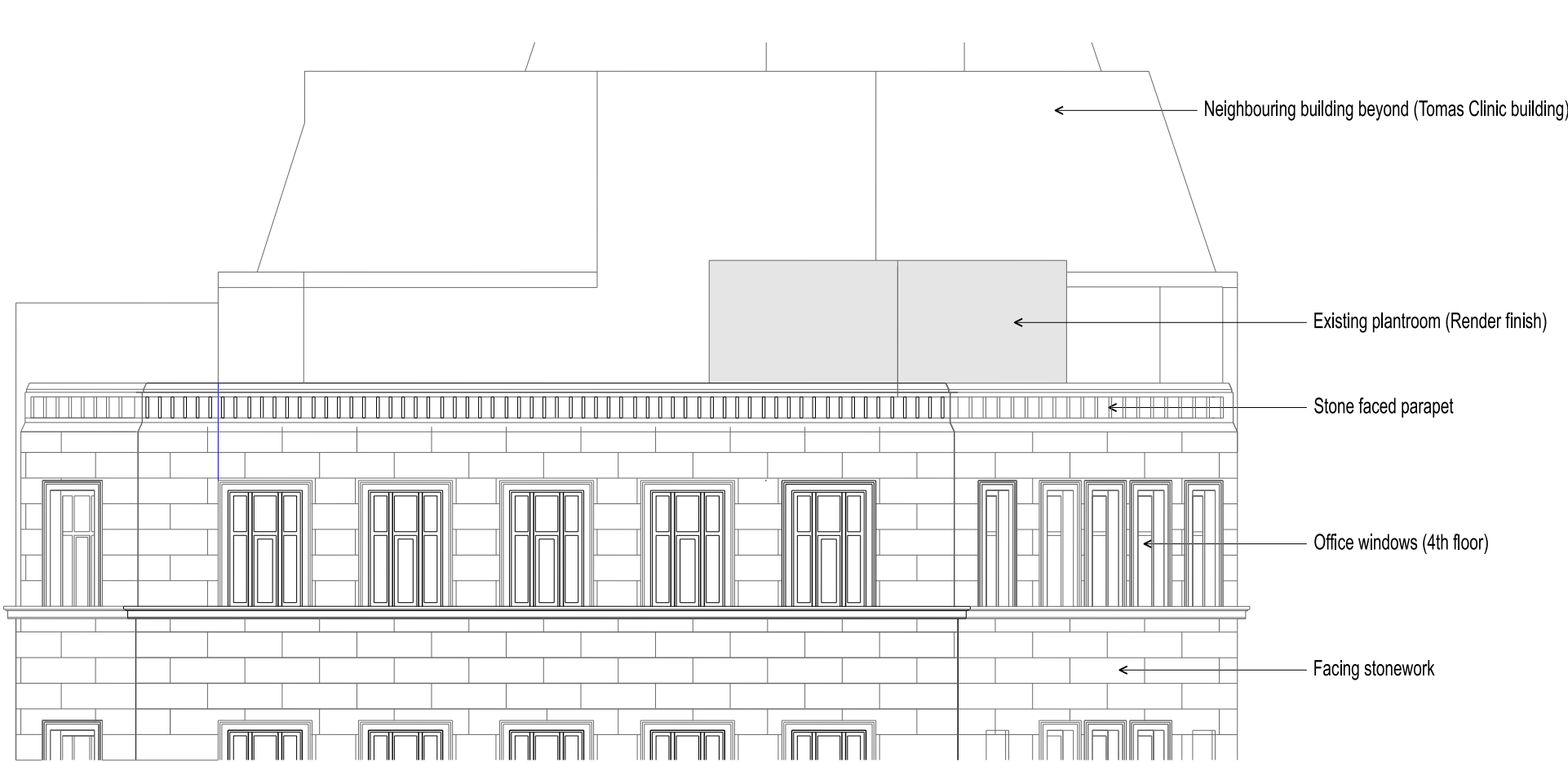
WATSON STREET ELEVATION - EXISTING 1:100
