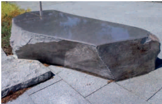
Naturally weathered granite boulders with cut and polished tops act as sculpture, natural play features and informal seating.
