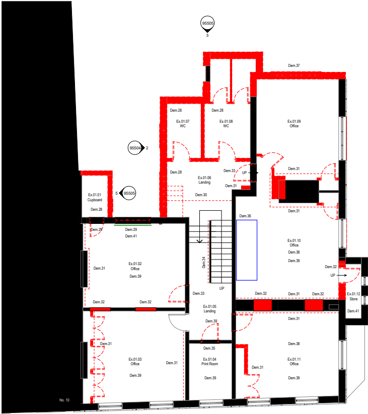
First Floor Demolition Plan
