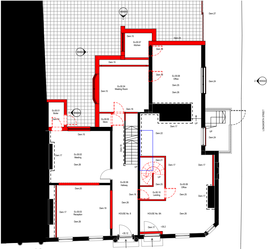
Ground Floor Demolition Plan
