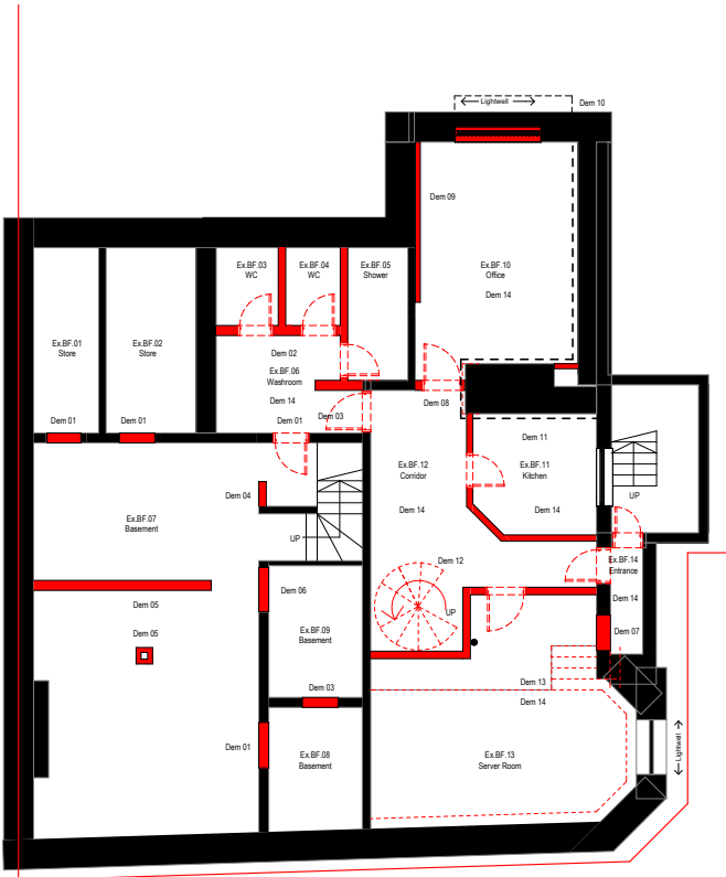
Basement Floor Demolition Plan
