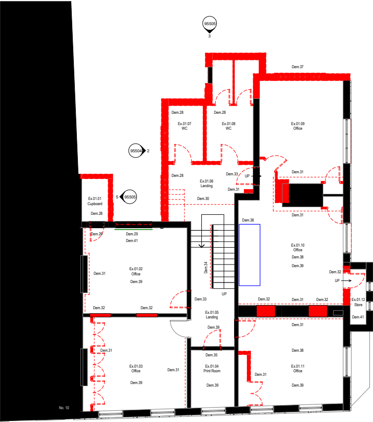
First Floor Demolition Plan
