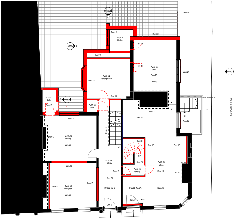
Ground Floor Demolition Plan
