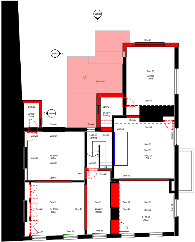
First Floor Demolition Plan
