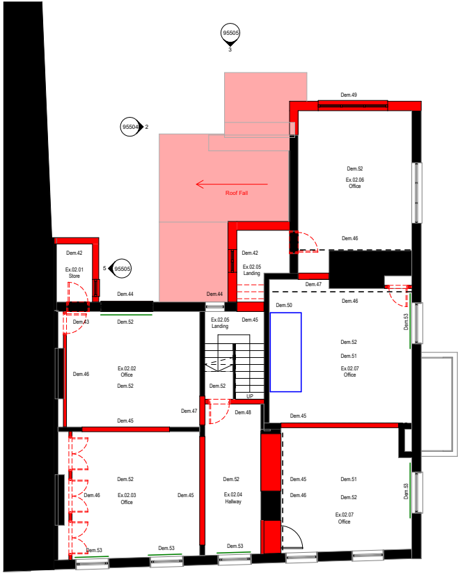
First Floor Demolition Plan
