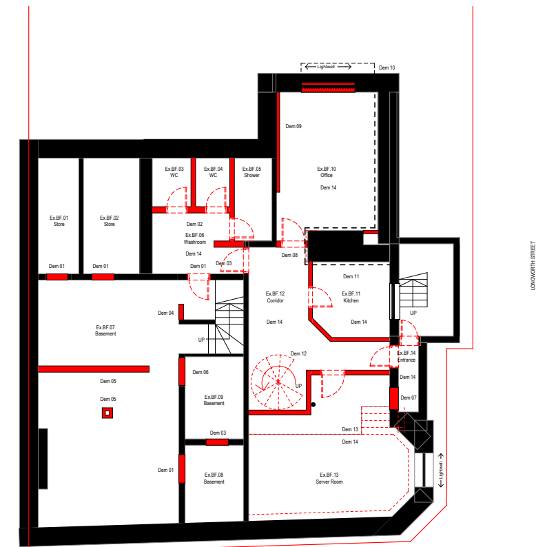
Basement Floor Demolition Plan
