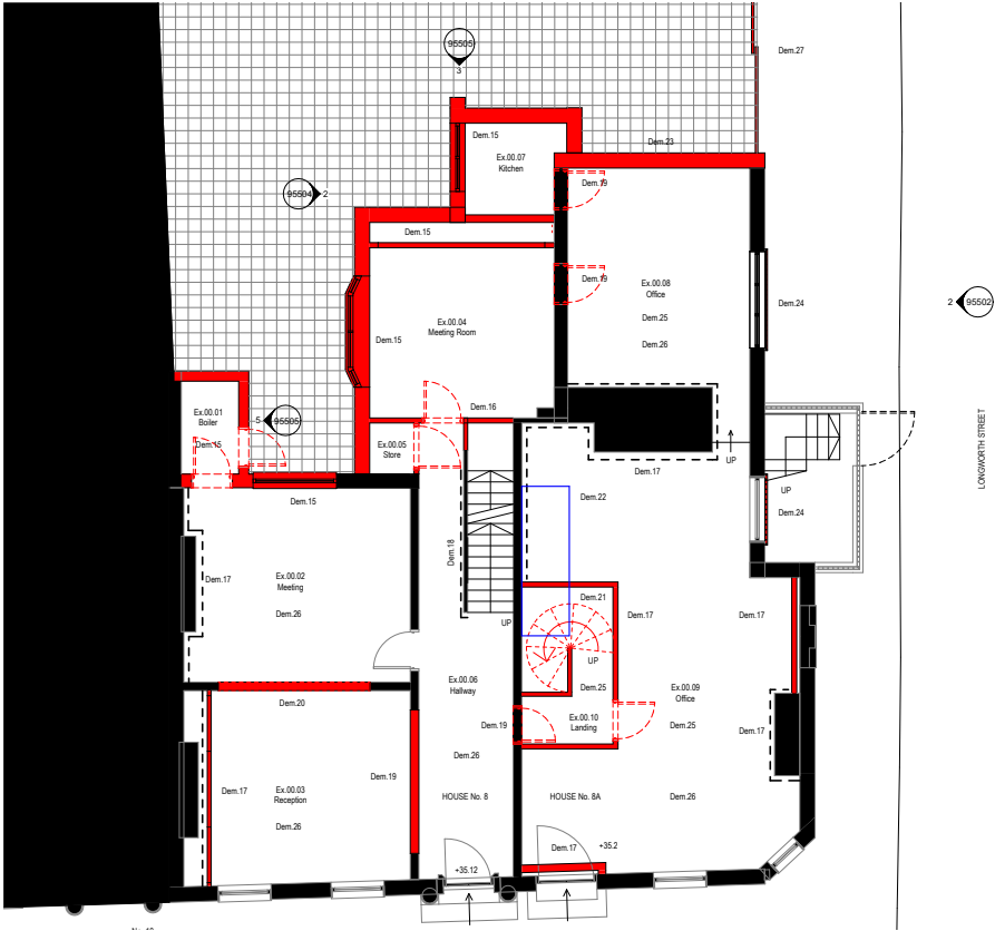
Ground Floor Demolition Plan
