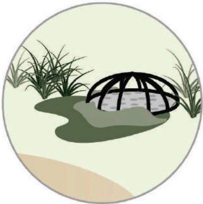
STORM DRAIN TO BE CLEANED OFTEN TO ENSURE ADEQUATE WATER FLOW
