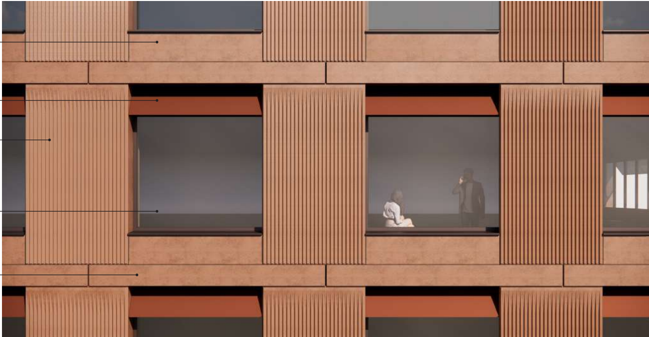
External elevation view of typical C1 western facade bay
