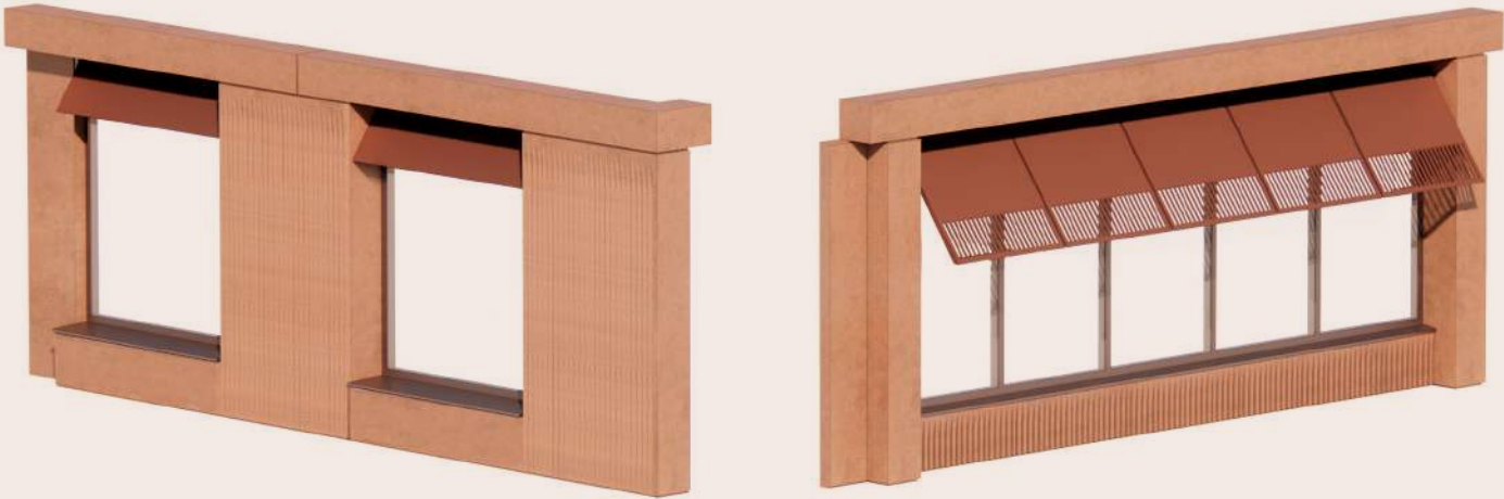
Glazing and metalwork installed offsite, assuring quality and robustness at key junctions
