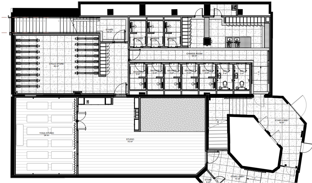
Figure 1 – Proposed basement plan (of works within scope of this application)
