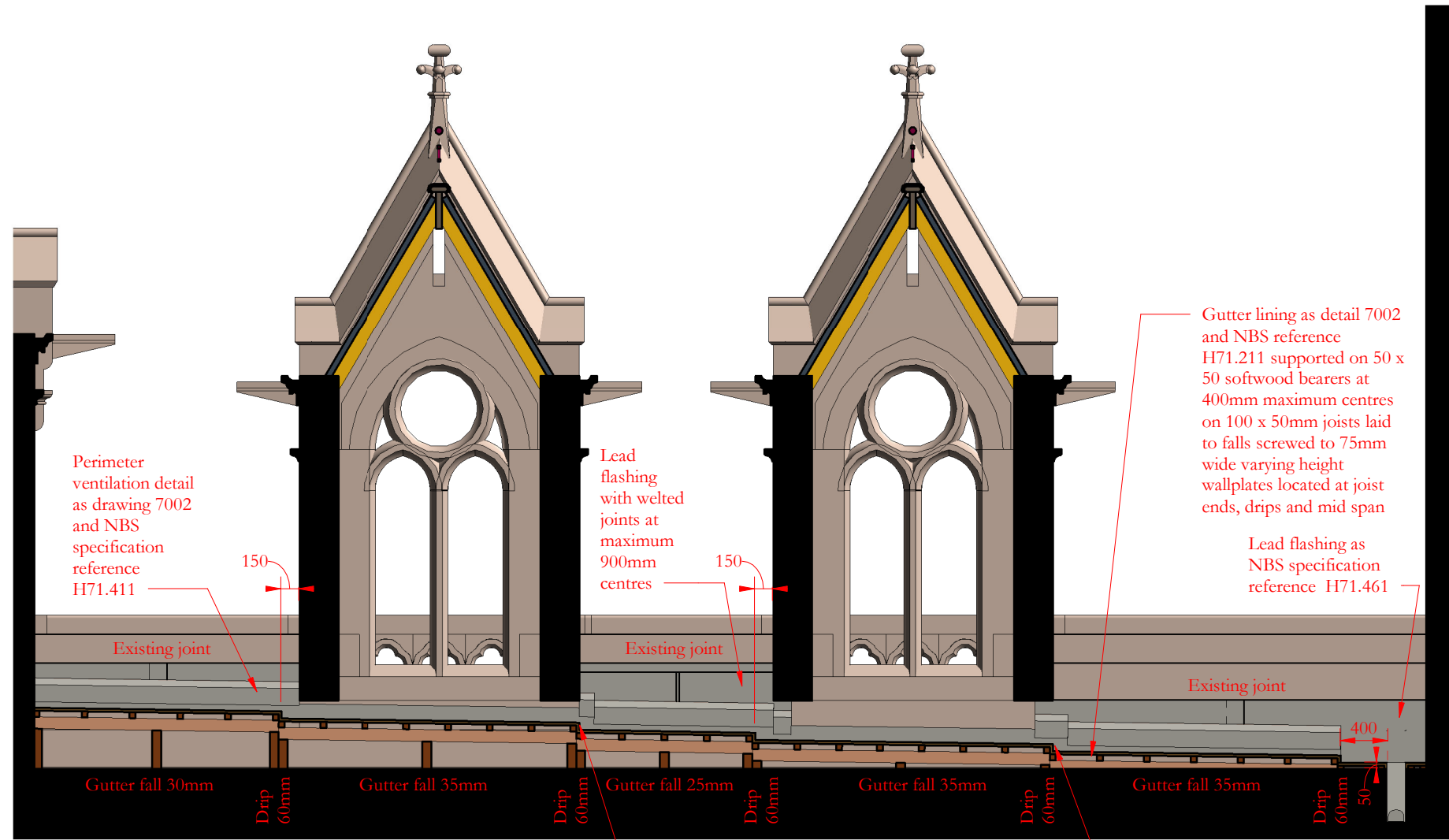
Gutter to Albert Square roof slope WR11 north
