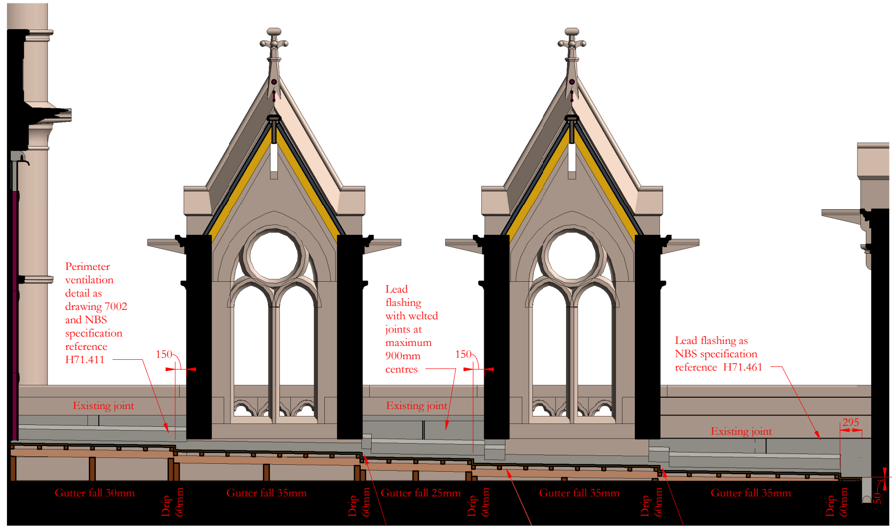
Gutter to Albert Square roof slope WR11 south
