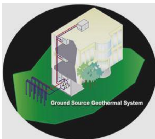
Fig. 5.1 – Ground-Source Heat Pump Installation
