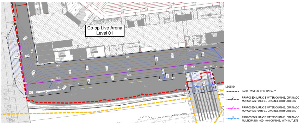
Figure 2—2 Existing Drainage & Levels
