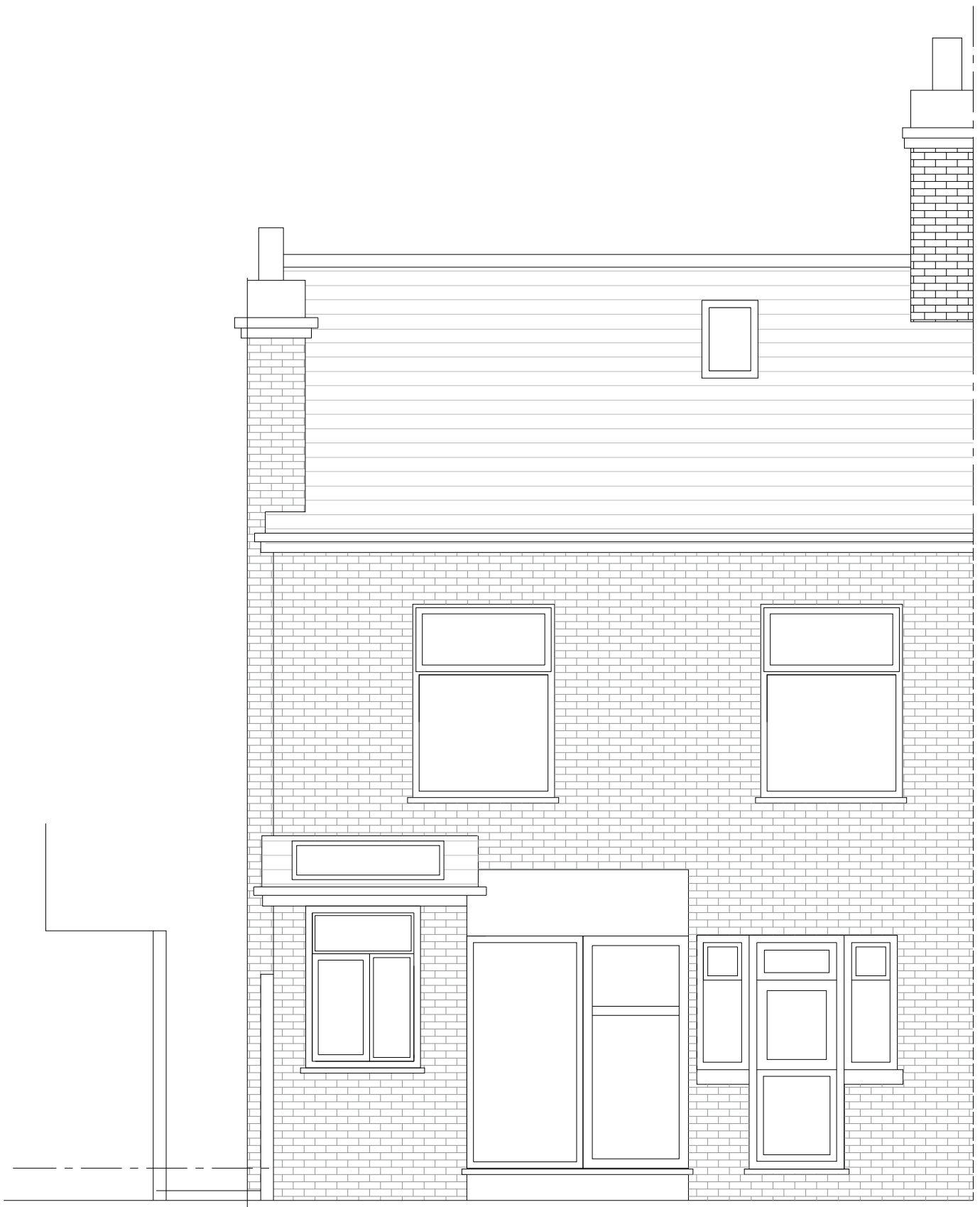
EXISTING REAR ELEVATION
