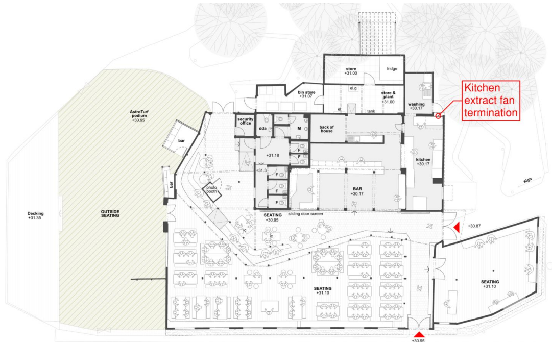
Figure 10 Kitchen extract fan termination location
