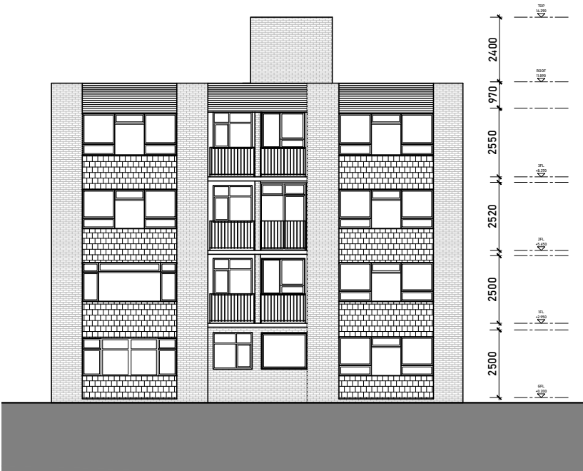
Existing Side (West) Elevation Scale 1:200 @ A3
