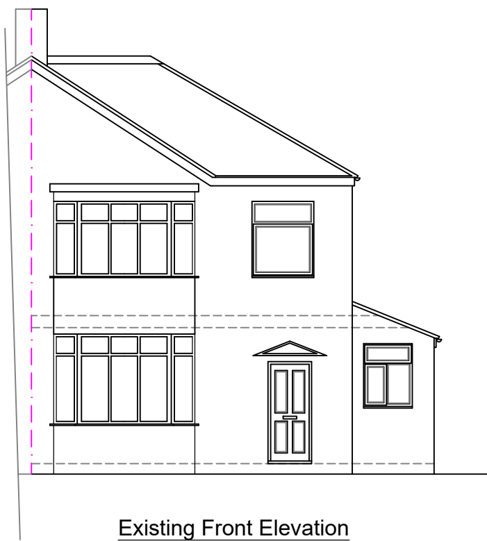
Existing Front Elevation
