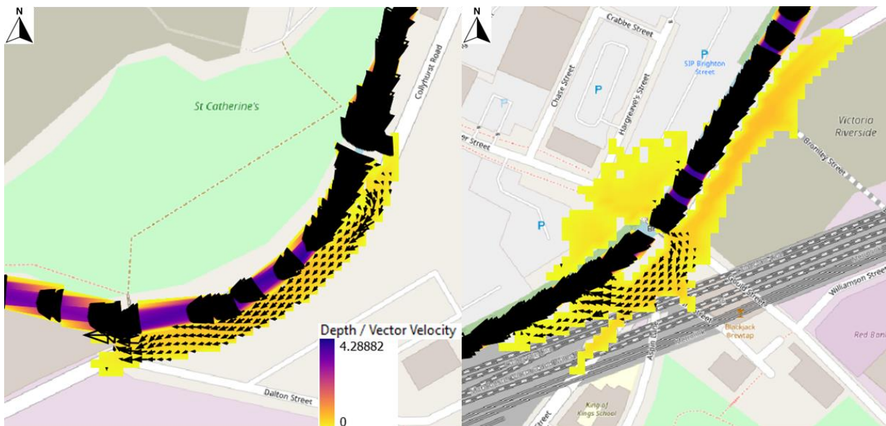
Figure 40: Key flood mechanisms around Collyhurst Weir and Union Bridge in the 20yr event, also demonstrative of flow paths in the 30yr event. The black arrows indicate vector velocity, showing flows leaving the channel downstream of Collyhurst Weir and upstream of Union Bridge
