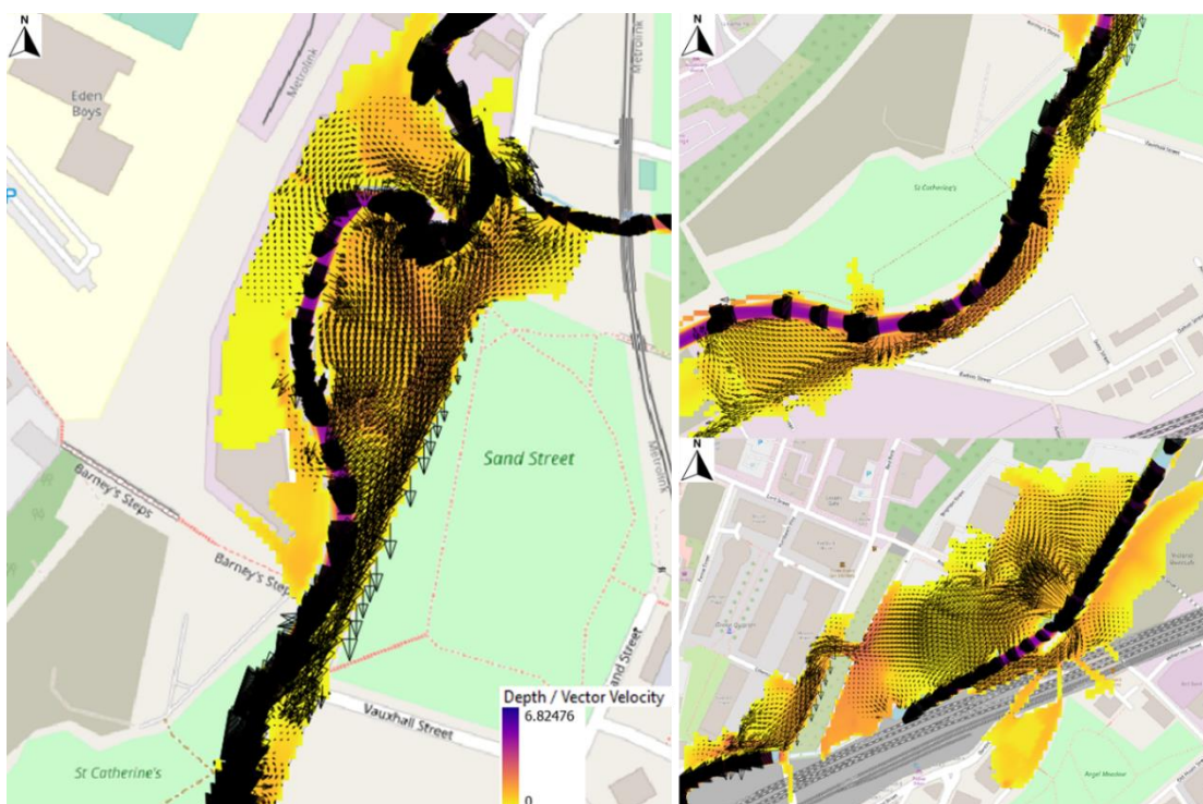
Figure 41: Key flood mechanisms around Collyhurst Weir and Union Bridge, in the 1000yr event, but also broadly applicable to the 100yr events with climate change allowances. Black arrows indicate vector velocity, clearly showing the flow along Collyhurst Road and Dantzie Street
