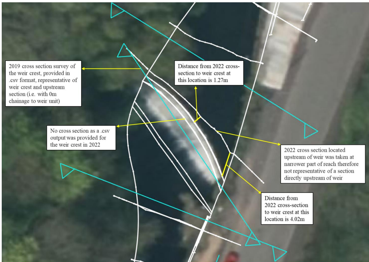
Figure 33: Location of Collyhurst Weir, and associated cross-sections surveyed in 2019 and 2022.
