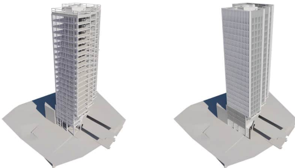
Figure 1 - SFS Model (Left) overlaid on Subcontractor Steel BIM model.
