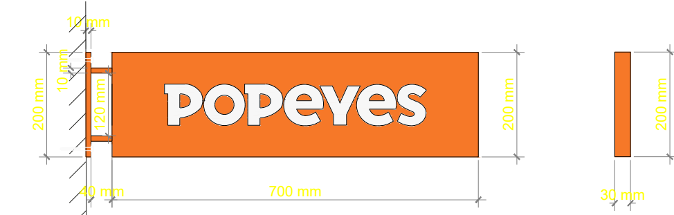
DETAIL 3 PROJECTION SIGN SECTION SCALE 1:10
