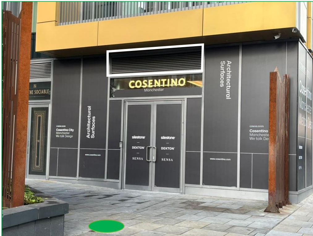
Figure 1: The proposed location of the air conditioning units (white rectangle), and the location of the sound level meter (green dot)
