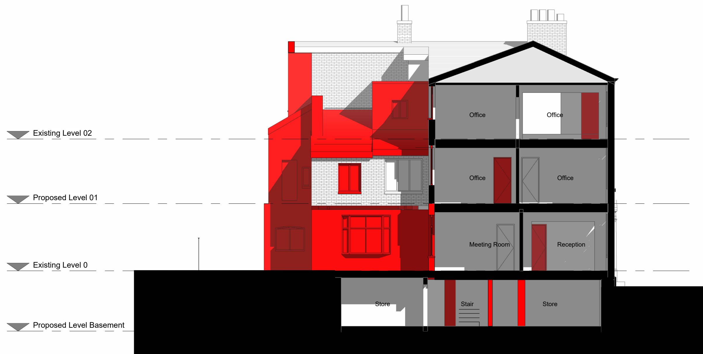
2 | B1 Existing West Elevation - Demolition 1 : 100
