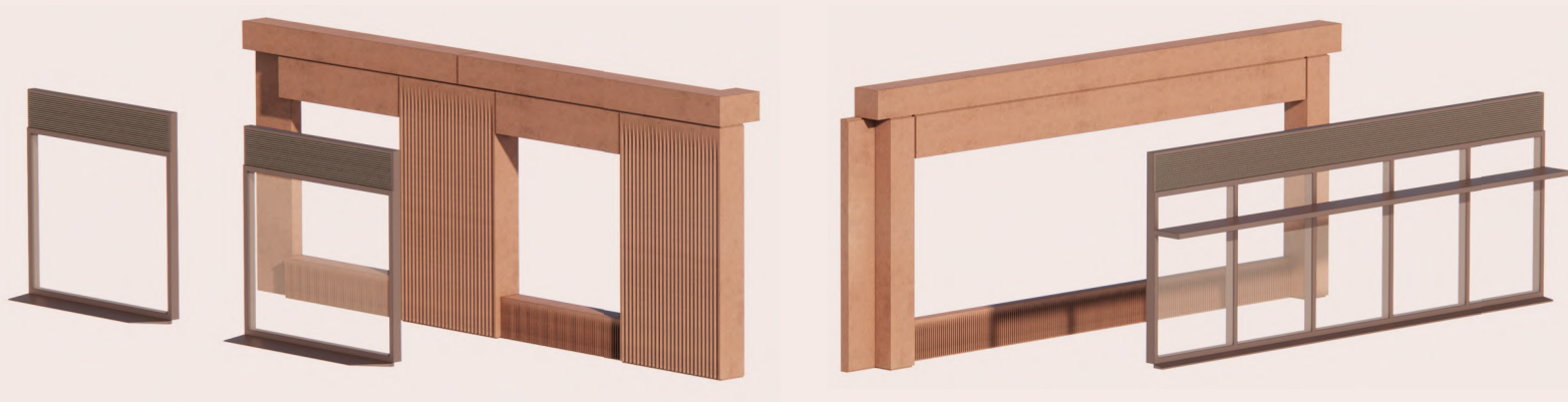
Glazing and metalwork including integrated continuous micro-profile performance louvres, installed offsite assuring quality and robustness at key junctions
