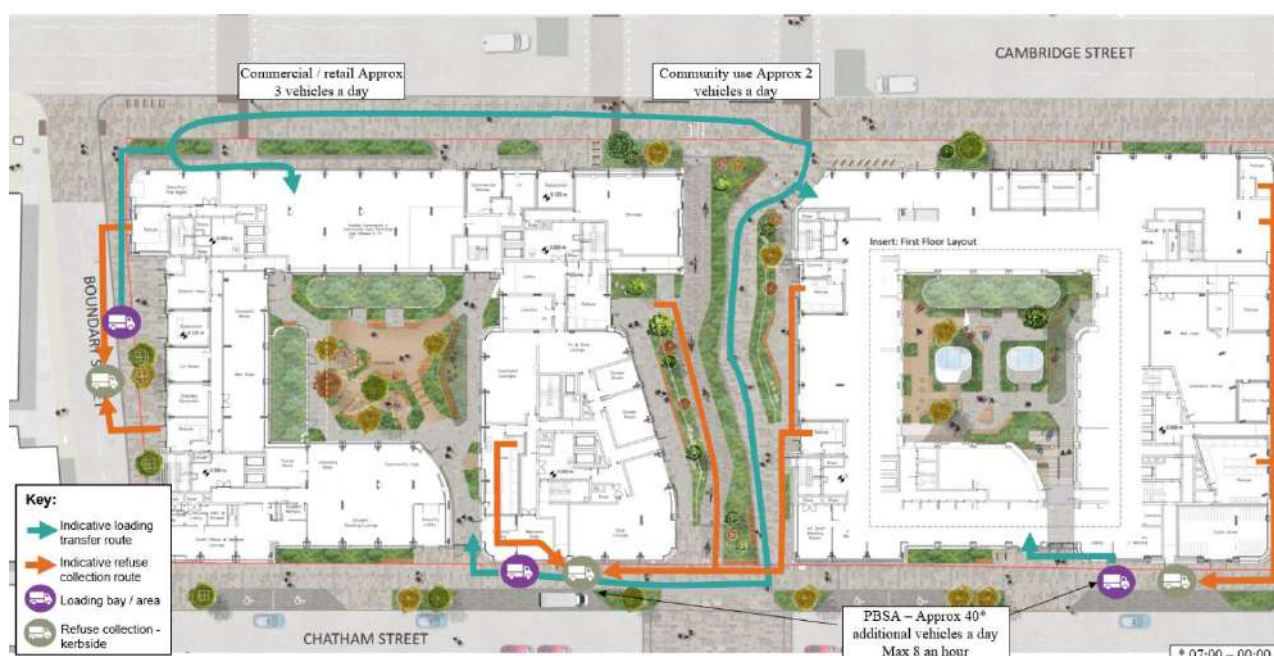
Figure 8: Servicing and Waste Collection arrangements
