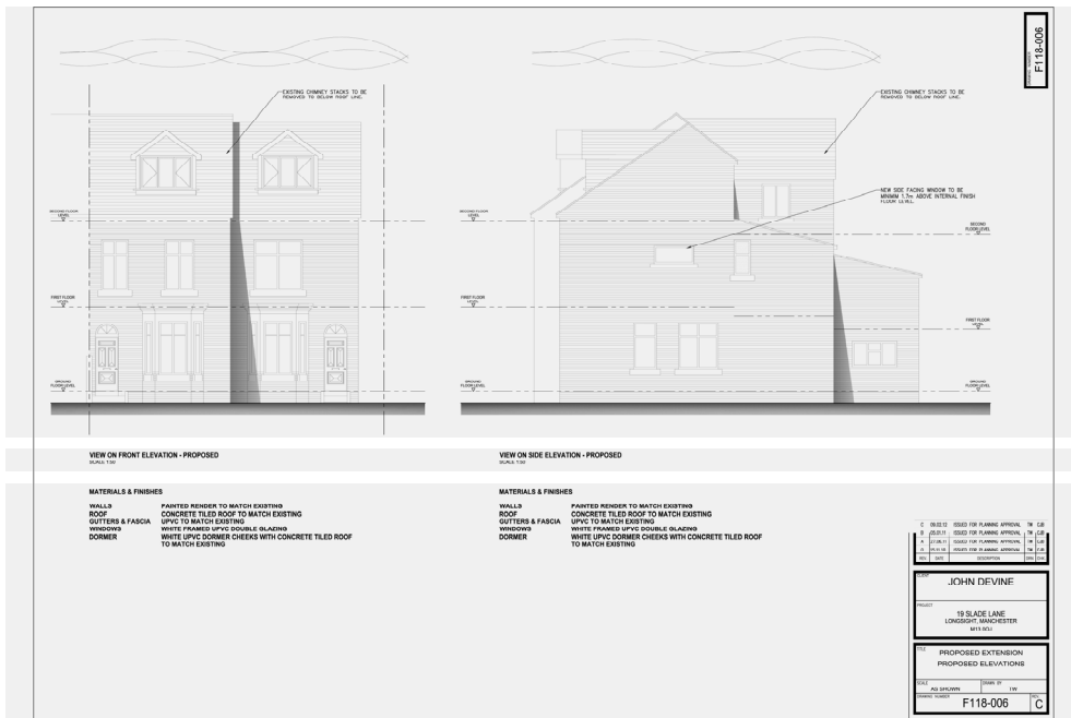
Fig. 3 Approved elevations for similar scheme application 096810/FO/2011/N2
