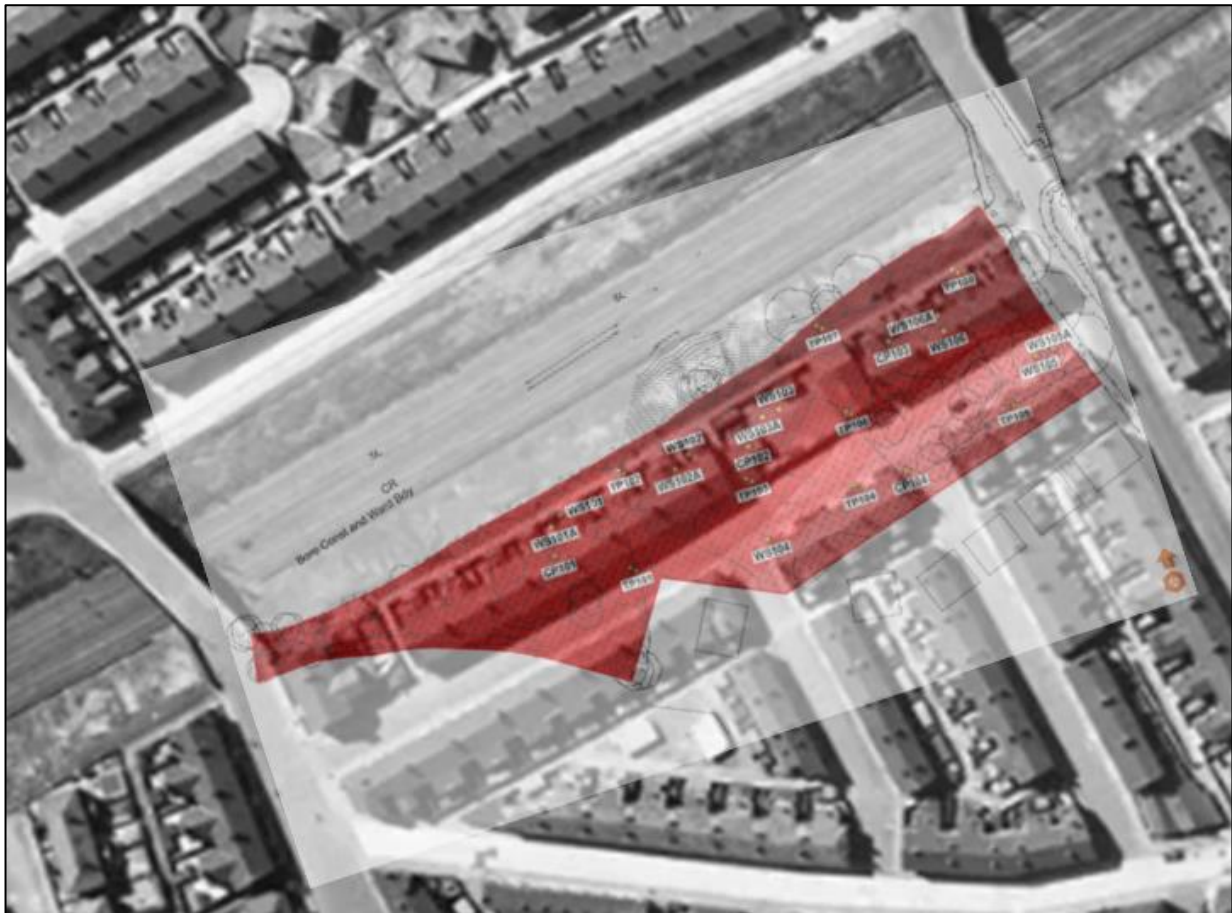
Figure 3.3-4: Exploratory holes plan Superimposed on 1946 RAF Photograph
