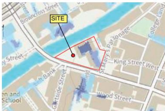
Figure 7.16 Environment Agency's Flooding from Surface Water Map (30 cm depth of water)
