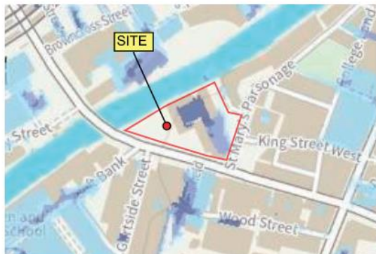
Figure 7.15 Environment Agency's Flooding from Surface Water Map (20 cm depth of water)
