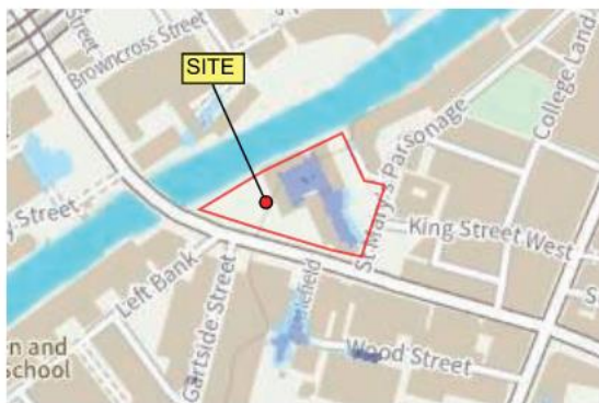
Figure 7.17 Environment Agency's Flooding from Surface Water Map (60 cm depth of water)
