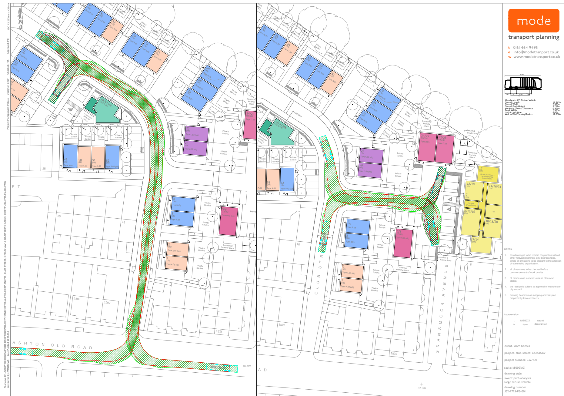
Proposed Site Plan showing vehicle tracking (provided by Mode Transport Planning)
