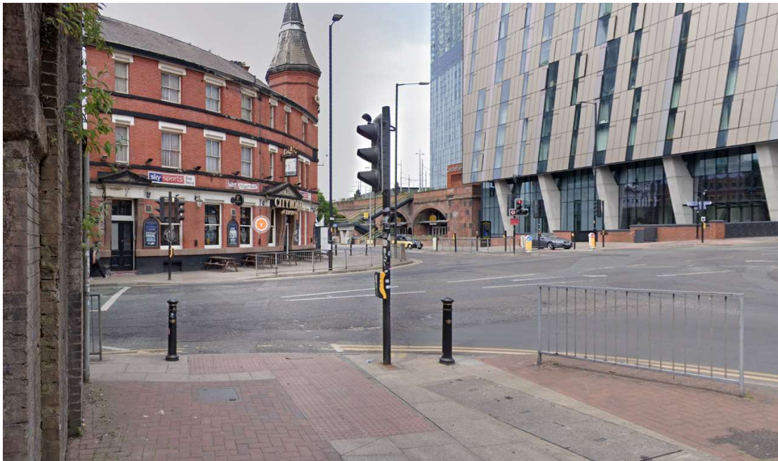
Figure 1 Medlock St/Whitworth Street Signal Pedestrian Crossing with Tactiles, Audible signal and Tactile Cone
