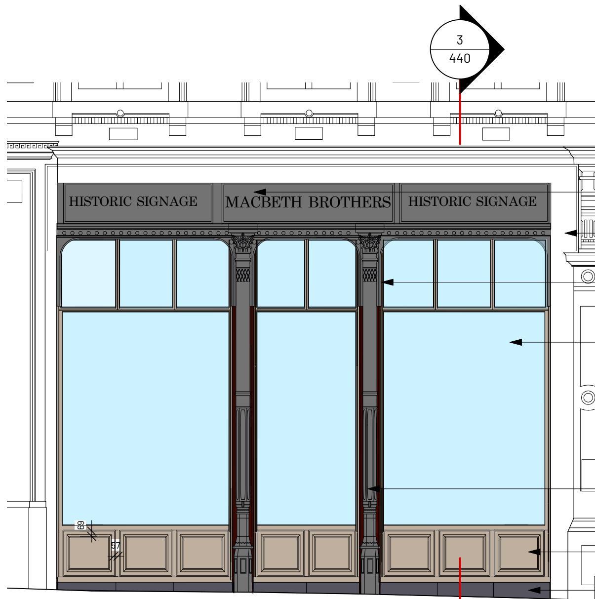
1 Proposed Shop Front Elevation Scale: 1:50
