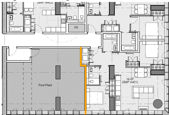
Image 3: Swimming Pool Plantroom-Bedroom wall on the 18th Floor of Building A
