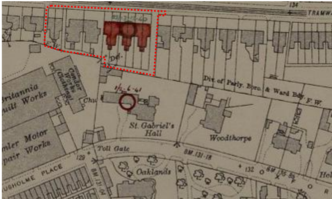
Figure 8 - 1932 OS (revised in 1941 to show wartime bomb damage) – This map illustrates the Site as it appeared in 1932 and shows that the six terraced houses to the eastern side of the Site were completely destroyed by a direct high explosive enemy bomb in December 1940 (shaded red).
