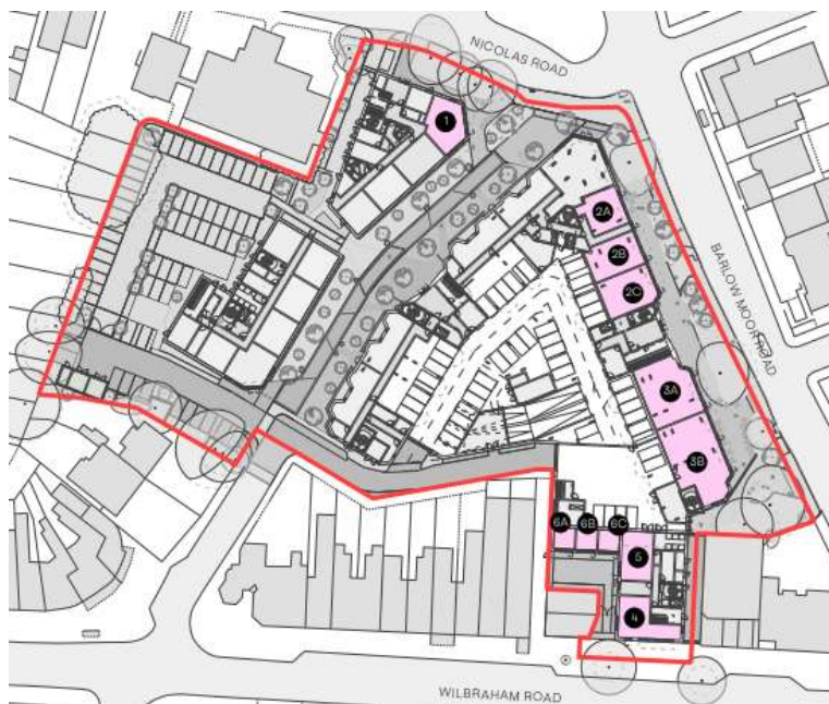
Figure 3-3: Ground Floor Retail Units
